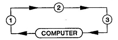
All messages move clockwise around the loop, relayed from one RPM1 to another. Each RPM1 picks off the messages addressed to it and relays responses or other messages onward.
