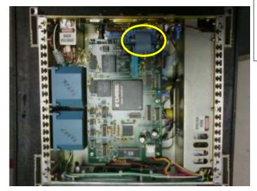
6. If your molbox has the MFC option then the MFC board will be above the driver board and it also has a ribbon cable from it to the back panel board. If so, you will probably have to disconnect the MFC board ribbon cable
