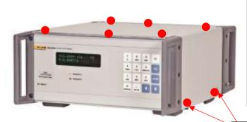
1. Remove the 10 screws that hold the cover on (molbox1+ with metal enclosure).
