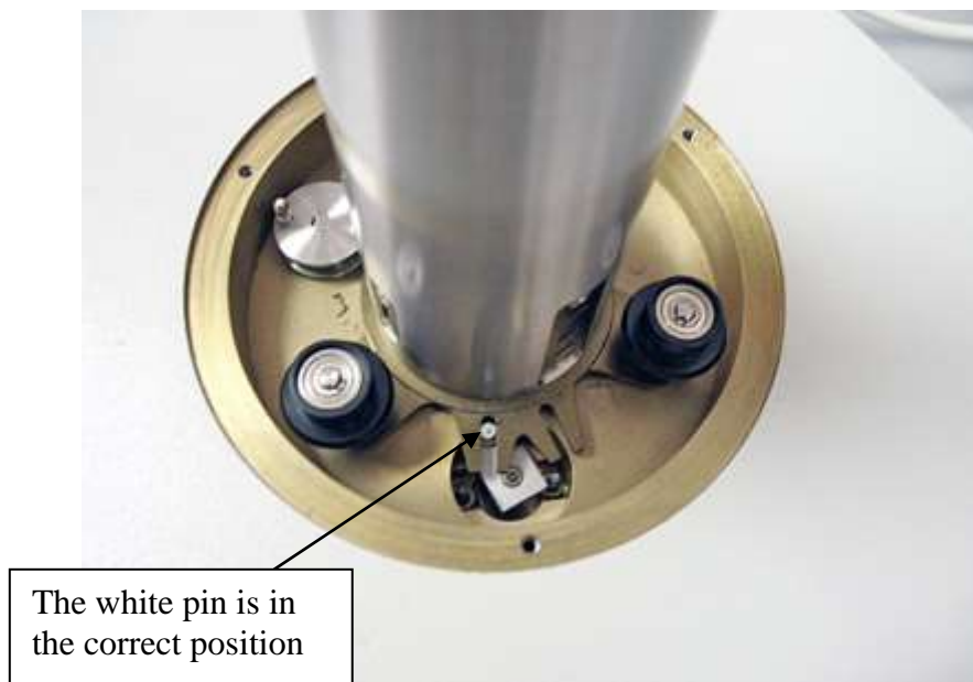
Figure 1: In a normal AutoRotate system, the white pin should be about 2 mm from the end of the slot when idle (solenoid is not engaged).
