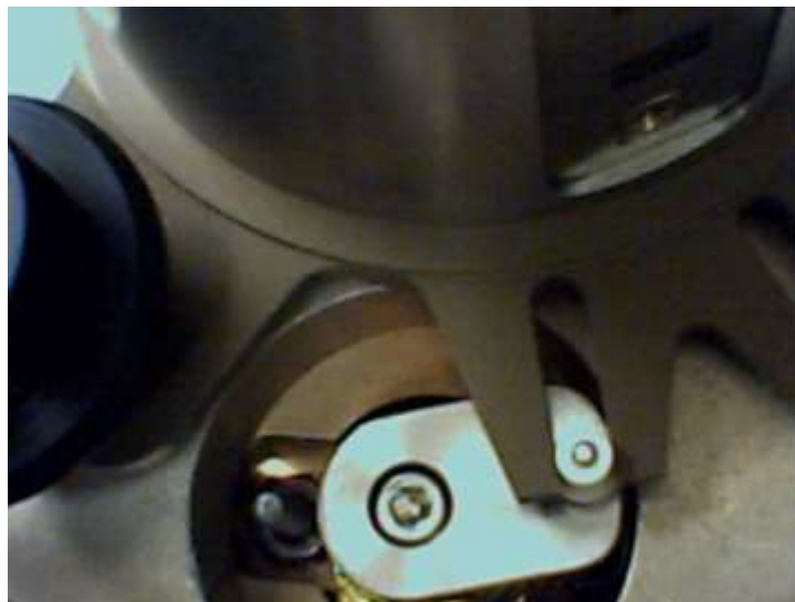
Figure 3: The solenoid is engaged and the white pin is in the correct position.
