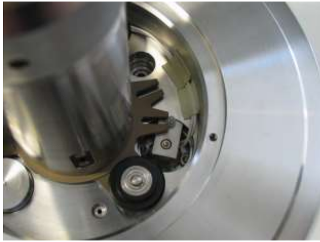
Figure 4: The solenoid is engaged and the white pin is in the wrong position
