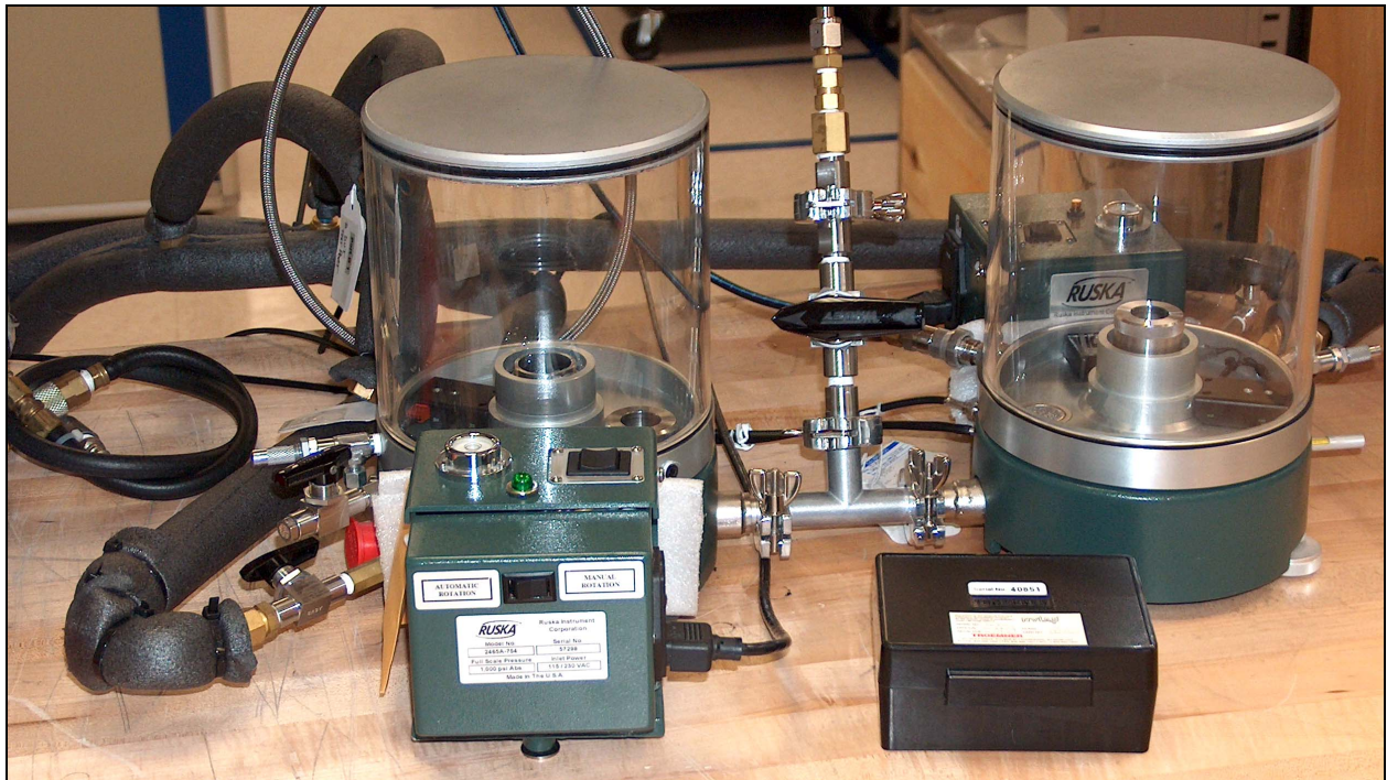
Two 2465 bases connected at vacuum port Note insulation on tubing and next to motor-case
