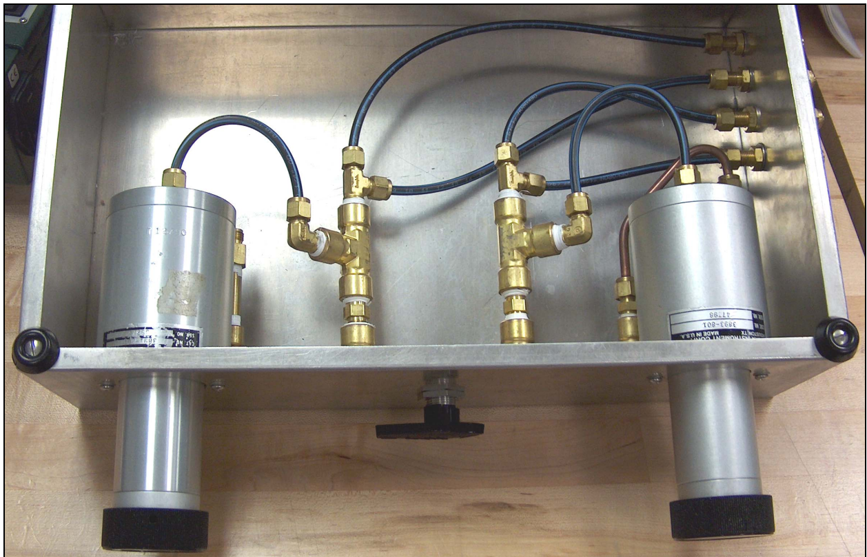
Two 3800-series volumetric pressure adjusters and ball valve for differential pressure isolation
