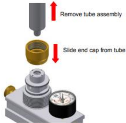
A2. This will release inner slide tube from non return valve at the base manifold end
