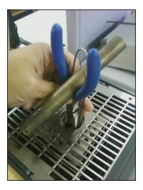
The insert could be lubricated with either WD-40 or ethanol. If WD-40 is used, after the insert is removed, clean the well and insert thoroughly and heat up to max temperature in very well ventilated area.
