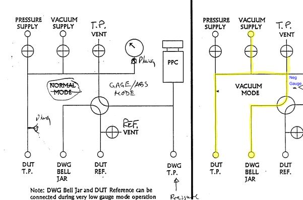
connected during very low gauge mode operation to reduce environmental influence. Vent valve on DUT REF. port replaces ball valve on 2465 base.
