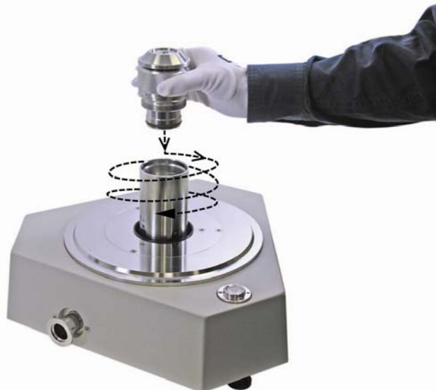
Figure 4. Piston-Cylinder Module Installation
