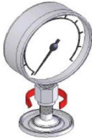
Figure 2-2. Making Pressure Connections
