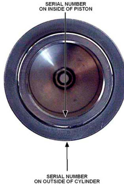
Figure 62. Alignment of the FPG piston in the cylinder
