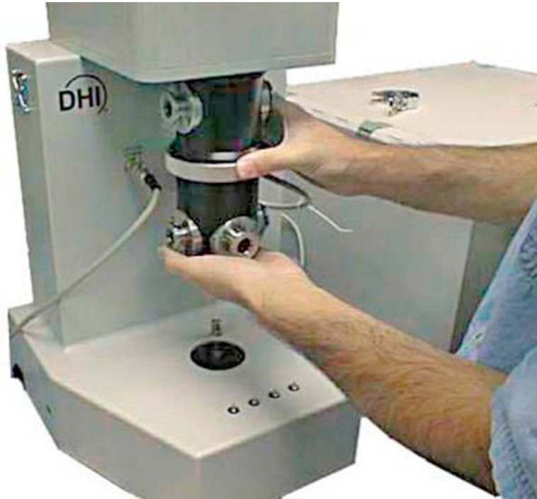
Figure 60. Removing the Mounting Post
