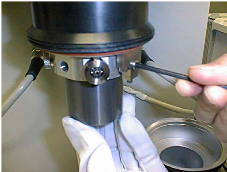
Figure 61. Removing the Piston
