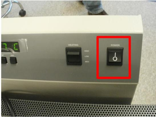
1 Turn OFF the power switch. Unplug the unit from the wall.
