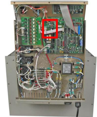
3 Locate the potentiometer on the analog board.
