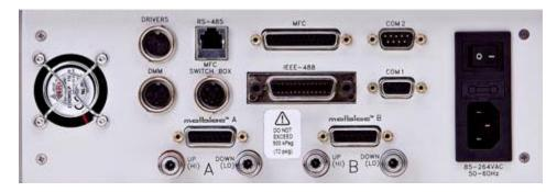
The DMM connector has 8 or 3 pins depending on the age of the molbox1 flow terminal. Only 2 of the pins are connected. This connection can be used to measure the voltage signal coming back from a MFC or MFM with an external DMM (that perhaps has better accuracy than the molbox1 internal MFC option circuit). The DMM connector is very rarely used.
