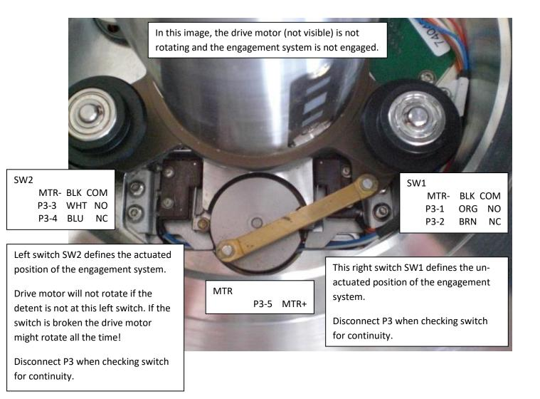
Note that this image is of a PG7601 piston gauge. PG7102, PG7202 and PG7302 piston gauges have the green PCB mounted on the bottom of the base.
